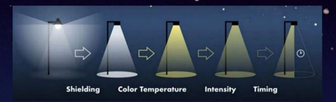
The above graphic by Remi Boucher illustrates progressive strategies that can be pursued, especially as technologies improve. The graphics below show the best examples of shielded lights, to point lighting, downward. Read more about Luminaire, Backlight, Uplight and Glare on our website on the back of this brochure.
